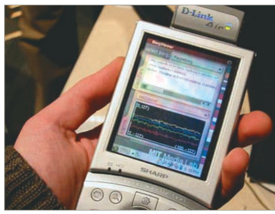
Figure 2. The GroupMedia system. The system, built around a Sharp Zaurus PDA, measures attraction signaling in dating and other social events. The system can also provide feedback to users and patch remote users in to interesting or socially important conversations. The interface in the image, which is still in the experimental stage, is a split screen of messages and biosignals from another user.
