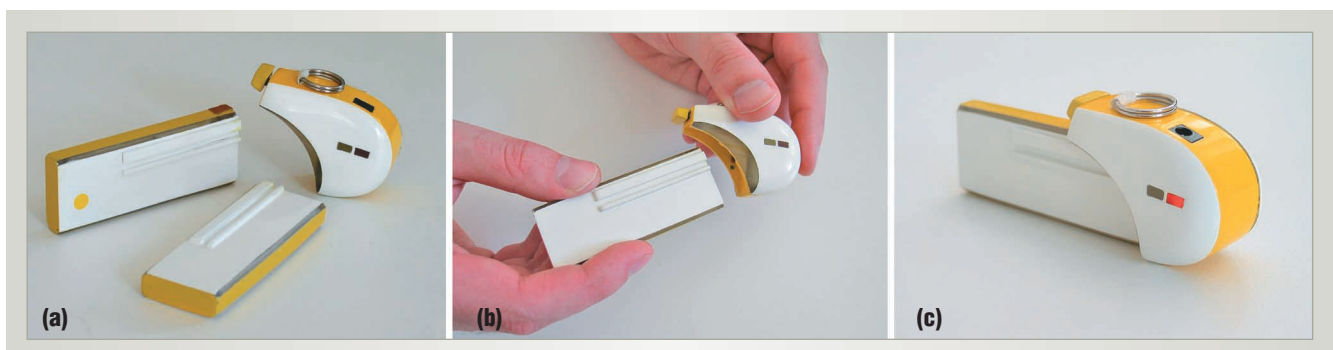
Figure 4. Personal Aura. (a) The reader module and two ID sticks, (b) connecting reader module and ID stick, and (c) an active Personal Aura.
